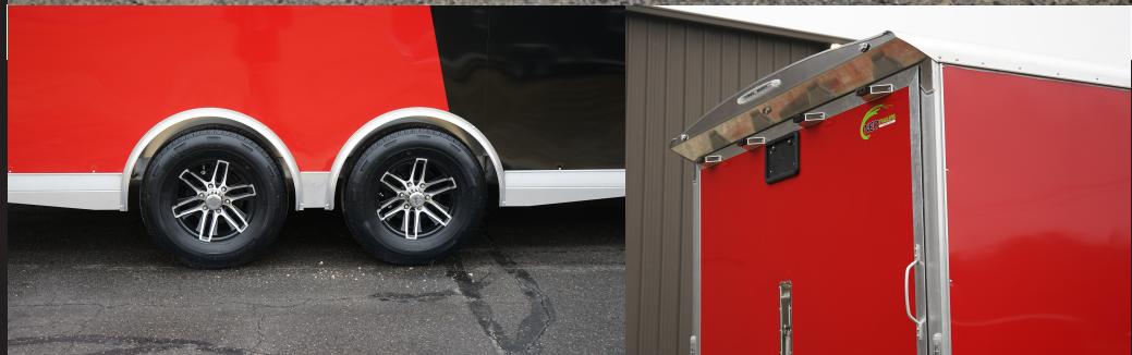
Upgraded 16" Wheels with 235 80 R16, Individual Aluminum Hoop Fenders
