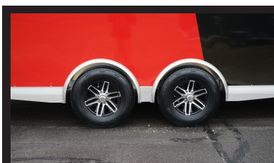
Big Rubber 16" Wheels with 235 80 R16, Individual Aluminum Hoop Fenders
